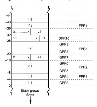
Figure 2-3 The organization of the parameter area of the stack
